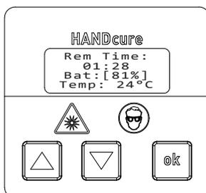
The HANDcure switches automatically off after the set exposure time has elapsed.
