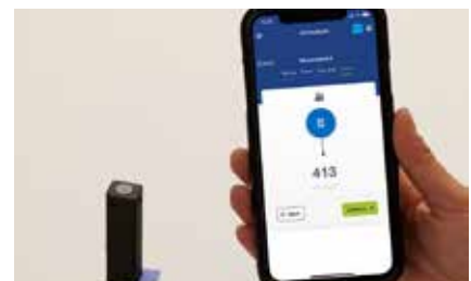
Take the measurement with the UV stick and transfer to the app via Bluetooth
