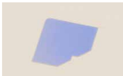
Irradiate the measuring strip with UV light; the measuring strip turns dark blue
