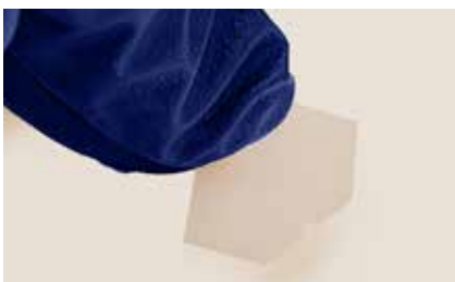
Use gloves and stick the measuring strip on a white (light) substrate
